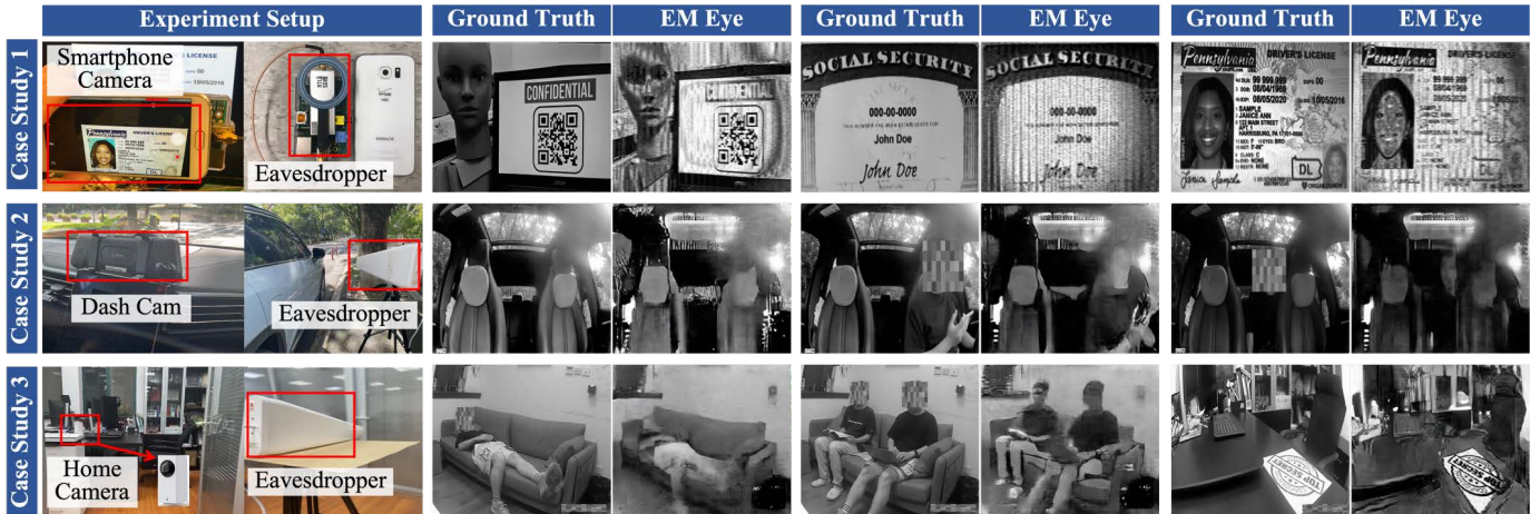
Fig. 13: Three case studies of how EM Eye poses eavesdropping threats against smartphones, dash cams, and home security cameras. For each case, the experimental setup and three examples of ground truths and eavesdropped images are shown.
