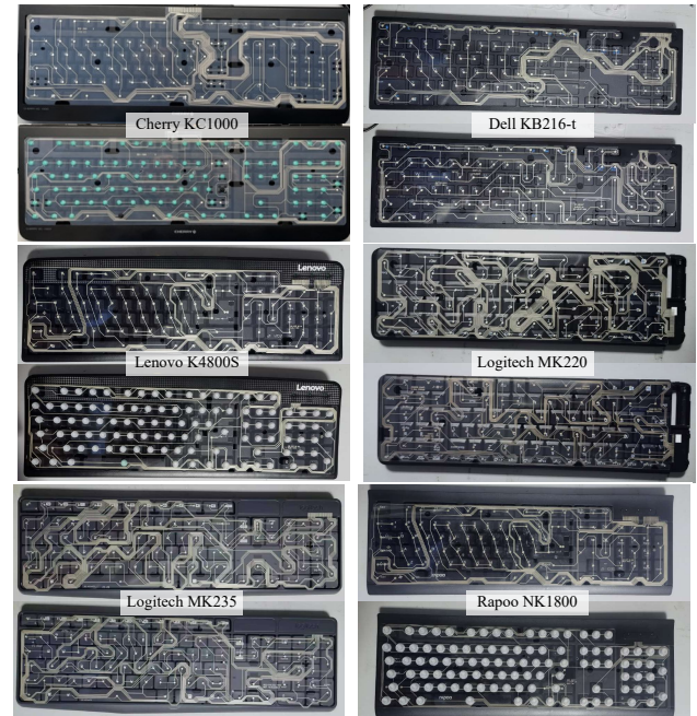
Fig. 19: Illustrations of the TX and RX traces on matrix circuits of 6 keyboards. We can find that these TX and RX traces are irregular and vary from keyboard vendor and model.
