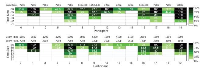
Fig. 8. The recognition results of textual reflections collected with local and Zoom-based remote video recordings from 20 user study participants. Participants 4, 14, and 3, 6, 10, 11 did not generate glass reflections that allow successful recognition due to problems of out-of-range viewing angles and very low light SNR respectively and are thus omitted from the figure.
