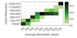
Fig. 13. Heat map of observed Zoom video resolutions under different low bandwidths that resulted in resolutions lower than 720p
