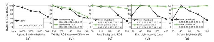
Fig. 7. Effects of impact factors evaluated by CWSSIM scores. The original score numbers are displayed along with the legend at the bottom, and we plot the ratio between each score and the highest score in each case as a percentage. Visualizations of the effects can be found in the appendix.
