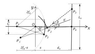
Fig. 12. The model of viewing angle.
